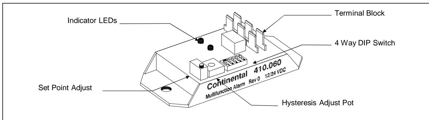
The 410.060 Multifunction Alarm is designed to give an alarm output when the reading on a particular gauge passes a predetermined level. The unit may be set to switch on either a falling or rising level for any type of gauge as long as the sensing unit is a variable resistance and the sender output is a variable voltage.
